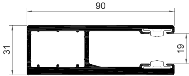
Figure 35: Cross-section side guide (PPW90) with a bottom slat
