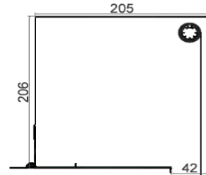
Figure 76: Cross-section roller shutter box (SP-E + MKT 205)
